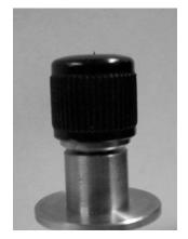
**C:** Screw the foot back onto the knife assembly until you see the blade protrude approximately 0.5 mm out of the foot's opening.
