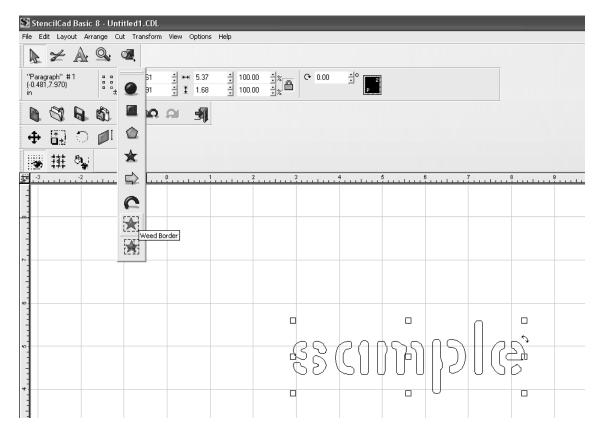
**B:** The size of the "Weed Border" can only be changed when it is being applied. This is done by using the dialog box on the upper left portion of the screen. Either use the up or down arrows or type in a value yourself. Note that when the size is changed, it is changed on all four sides of the stencil.
